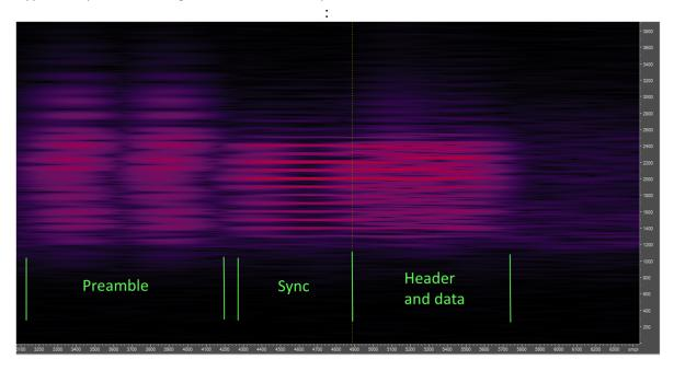
The transmitter encodes the data provided with 8-channel OFDM and PSK (QAM-4) for every channel, adds preamble (two following extended Barker's code sequences), creates synchronization sequence, adds a header (consisting of data type, length, data CRC, and header CRC), and then adds encoded data. In the end, wave data is sent to the DAC and then played by the speaker.
