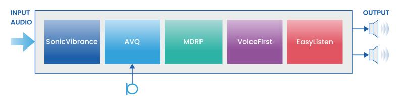
SonicVibrance<sup>™</sup>: Improving the perceived quality by optimizing the stereo image for a device, adapting the frequency content to the user's preferences and boosting the bass without overloading the speakers.
