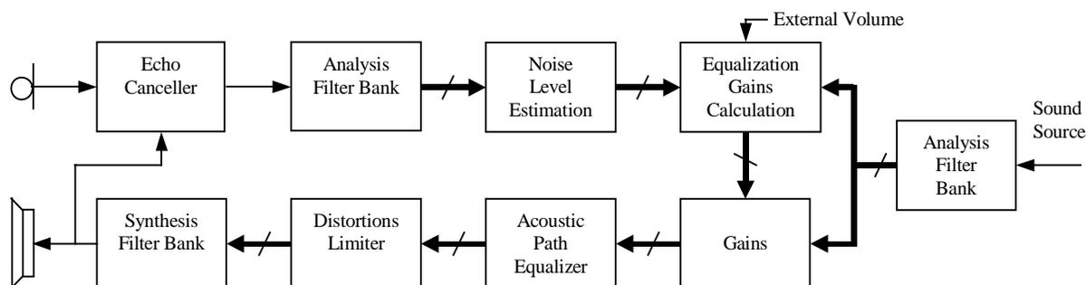
Fig. 1. A scheme of a sound equalizer in a noisy environment
